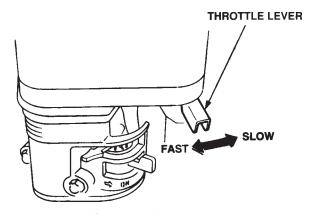
Figure 14. Throttle Lever
